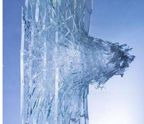
When a pane of glass breaks, small fragments of glass are ejected backwards as well as forwards, typically for up to 2 or 3 metres. These fragments can land and become lodged in the tools, clothing and/or hair of the person breaking the window. So not only is it possible to identify if a suspect was present at the crime scene, you can even determine from which side a window was broken.
